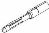
PIN CONTACT 3 TINE SPRING MEMBER, CRIMP
