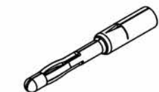
PIN CONTACT 3 TINE SPRING MEMBER, CRIMP
