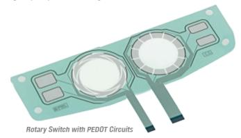
Figure 1: Molex PEDOT enables the inexpensive production of flexible, transparent sensors, enabling keypad backlighting on curved surfaces.
