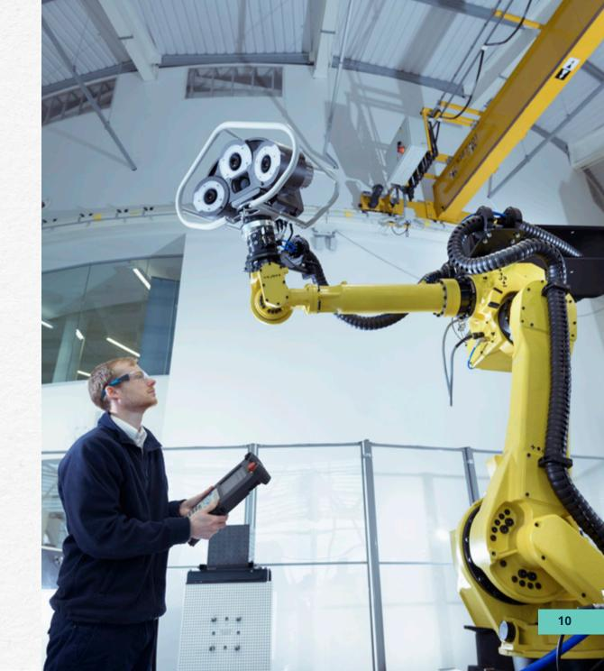
For example, torque sensors, which measure rotational force, now permit cobots to detect minute variations in pressure and force, enabling precise adjustments in real time. This is especially critical in industries like electronics, where even the smallest deviation can affect product quality. Machine vision and, in some cases, LiDAR, allow cobots to map and navigate complex industrial environments autonomously, ensuring high productivity and safety, even as conditions change.
