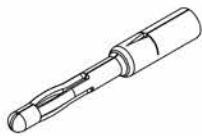
PIN CONTACT 3 TINE SPRING MEMBER, CRIMP
